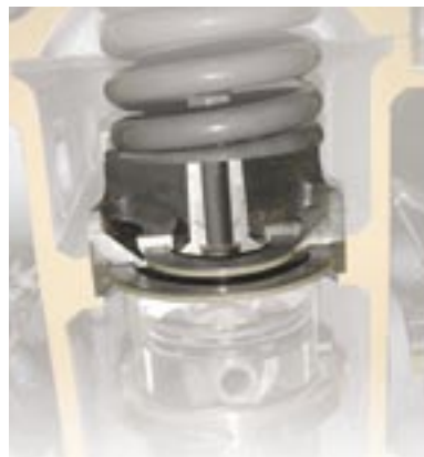
Figure 2: Construction of a cylinder head with ring valves
